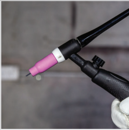
(1) Make sure the front end parts of the TIG torch are correctly assembled, use the correct size and type of tungsten electrode for the job, the tungsten electrode requires a sharpened point for DC welding.
