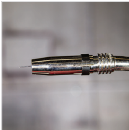
(13) Fit the gas nozzle to the torch head.
