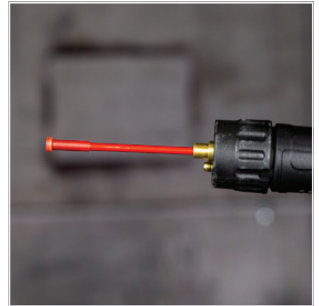
(3) Carefully pull out and completely remove the liner
